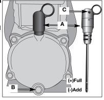
**NOTE:** Use an oil specifically formulated for use in an air compressor, such as Porter-Cable PAS1 air compressor oil. Oil may be found at the store where the air compressor was purchased.
